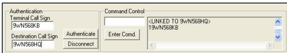
Figure 5.28: Linked message will appear in command control column when the link is established.
