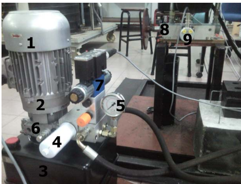
Figure 4. Experimental workbench for electro-hydraulic system. 1-electric motor; 2-pump; 3-tank; 4-filter; 5-pressure gauge; 6-relief valve; 7-proportional valve; 8-hydraulic actuator; 9-wire displacement sensor
