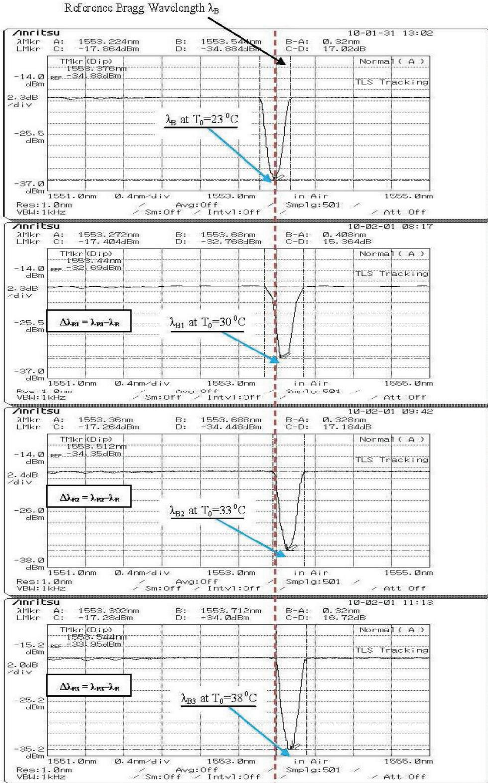
Fig 3: FBG Transmission Spectra
