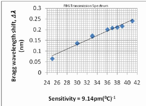
Fig 5: Transmission spectrum
