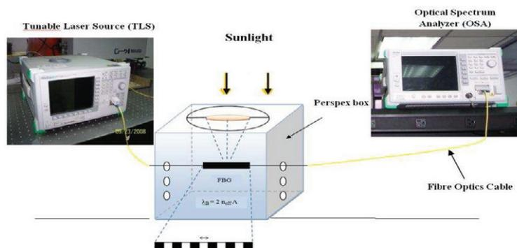
Figure 2: The experimental set-up for the transmission wavelength spectrum
