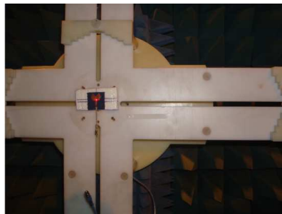
Figure 16. Snapshot of radiation pattern measurement setup inside an anechoic chamber for antenna #1 design.
