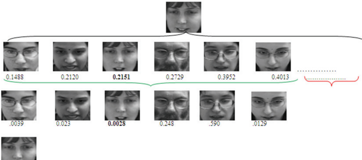
Fig. 5: Case-I: first row contain probe image, 2nd row contains the Euclidian distance computed on LDA, and row 3 contains the CSLDA results computed on adaptive new database as a result of row 2, whereas row 4 the recognized results
