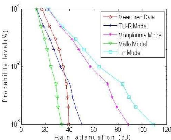
**Figure 2.** Comparison of rain attenuation CCDF at 15 GHz.
