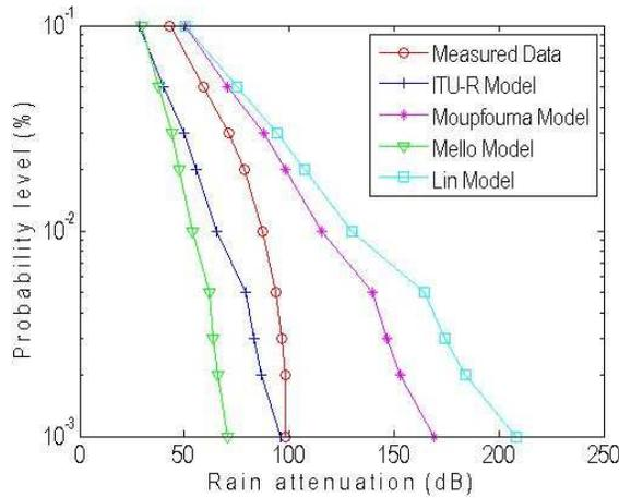
**Figure 3.** Comparison of rain attenuation CCDF at 26 GHz.
