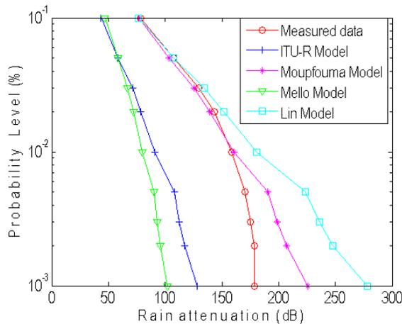
**Figure 4.** Comparison of rain attenuation CCDF at 38 GHz.
