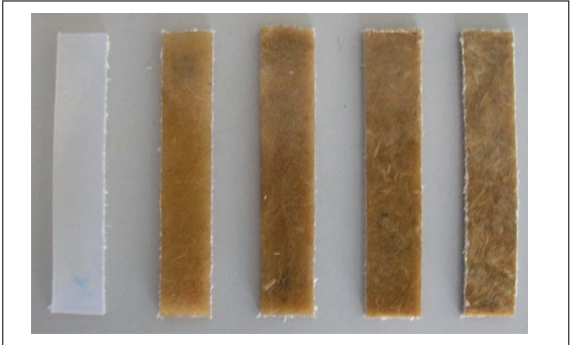
Figure 3.12: Impact Testing Specimens for Various wt% of PALF Reinforced in PP
