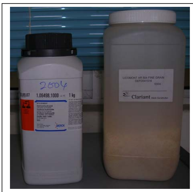
Figure 3.3: Left is the Natrium Hydroxide Used for Chemical Treatment while the Right is the Coupling Agent – Licomont AR504 Used
