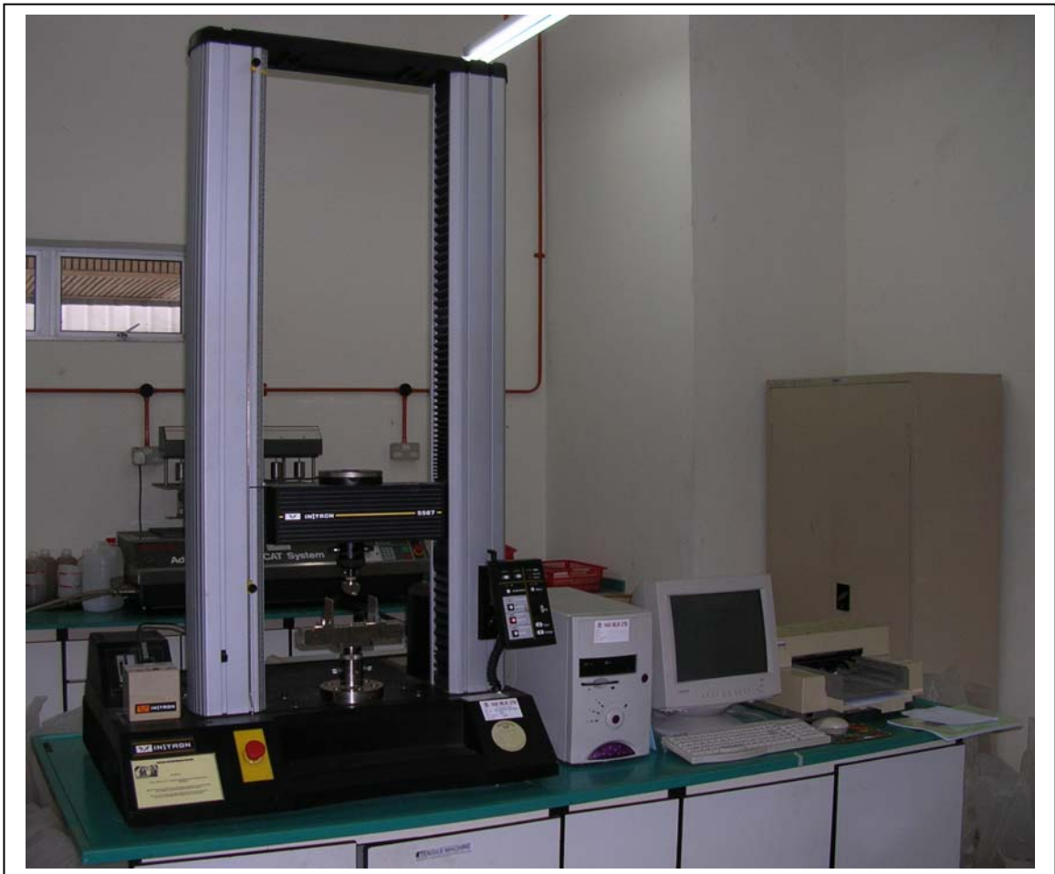
Figure 3.7: Universal Testing Machine - UTM (Instron 5567) for Tensile and Flexural Testing
