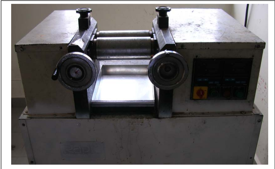
Figure 3.1: Raptic Two-roll Mill Machine Used for Remove Water and Composite Compounding
