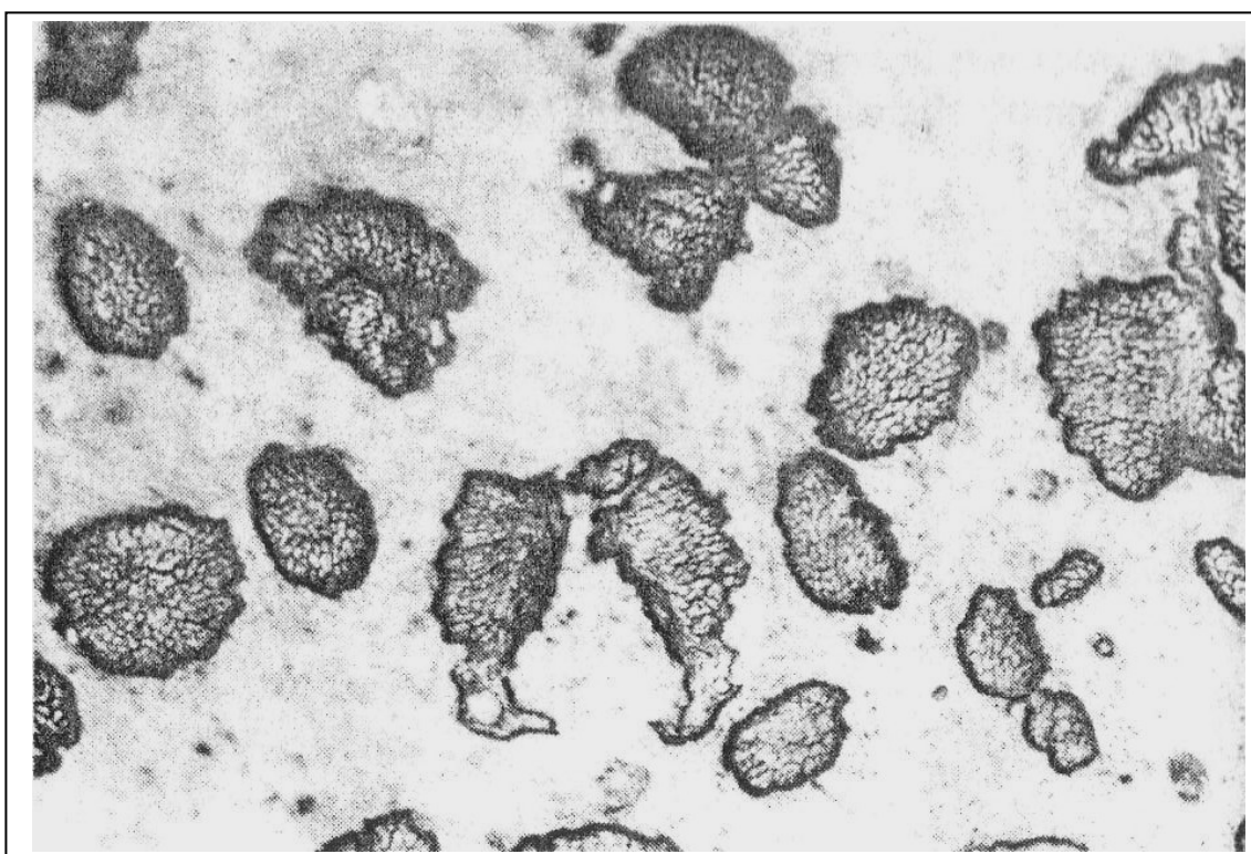
Figure 2.6: Optical Micrograph of Cross Section of PALF ( \times 160 magnification) (Mukherjee et al. , 1986)
