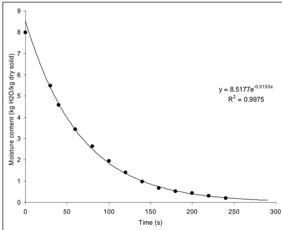
Fig. 2. Moisture content curve for microwave power 380W
