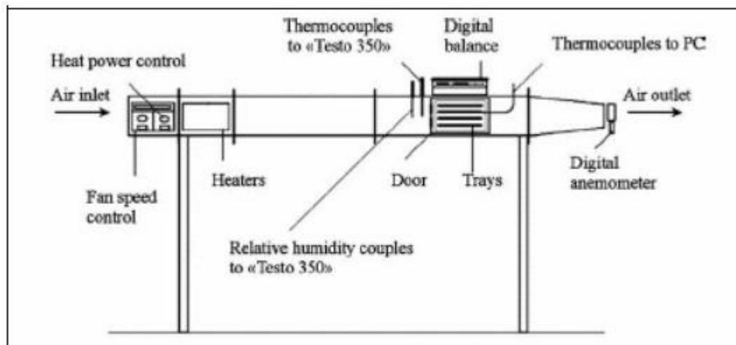
**Fig. 6.** Schematic diagram of the convection drying equipment
