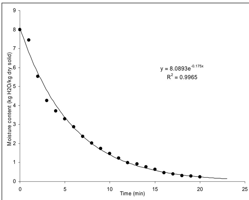
Fig. 1. Moisture content curve for microwave power 110W
