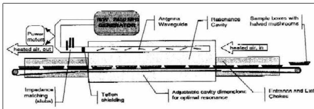
**Fig. 3.** Schematic representation of microwave drying unit
