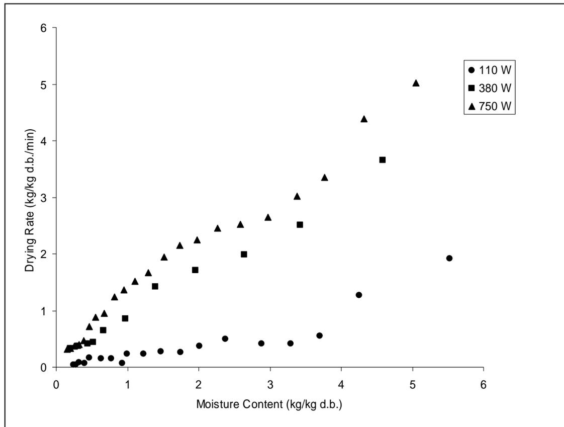
Fig. 4. Drying rate curves for different microwave power intensities
