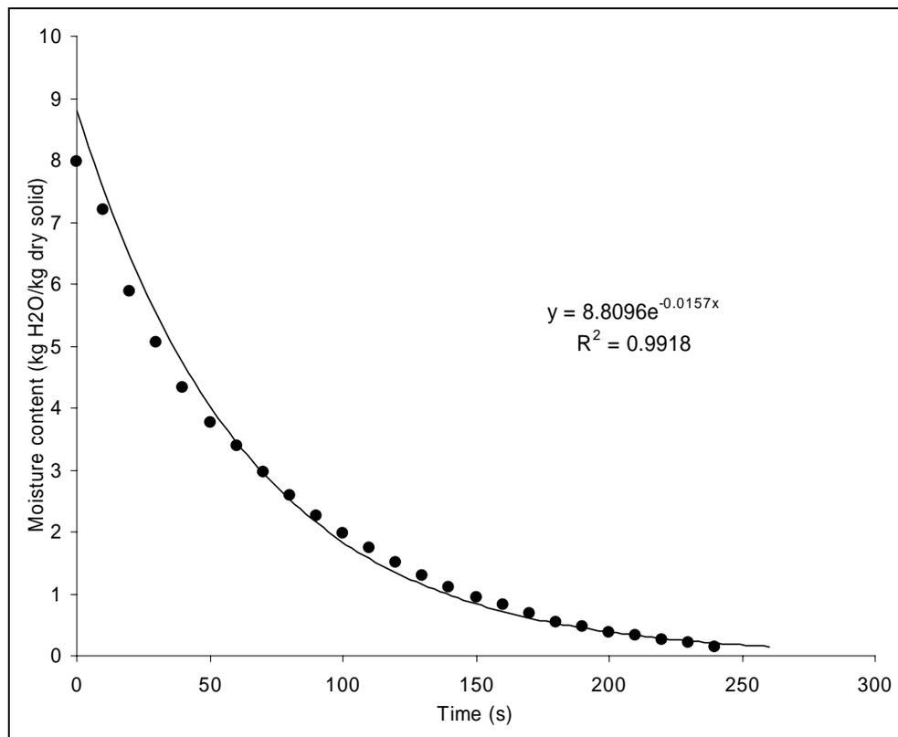
Fig. 3. Moisture content curve for microwave power 750W
