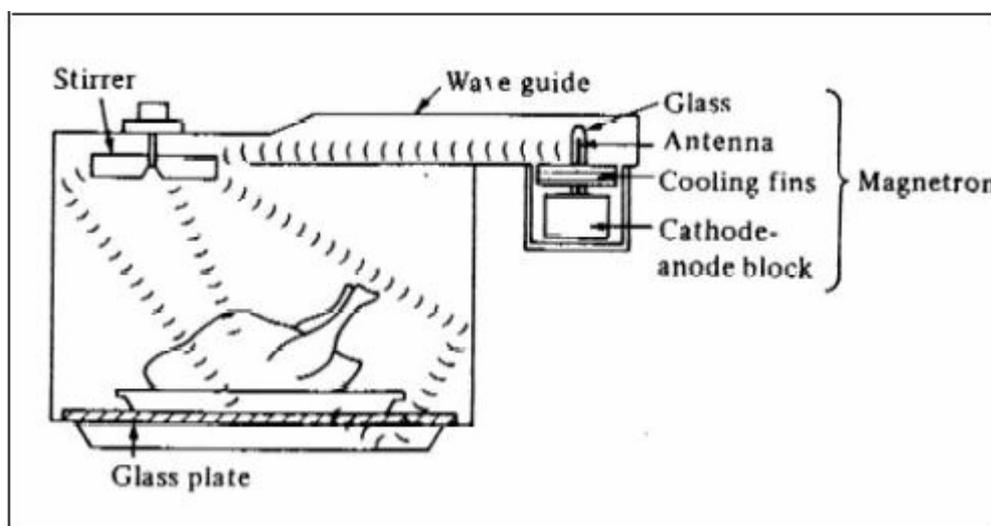
**Fig. 2.** Microwave oven drying unit
