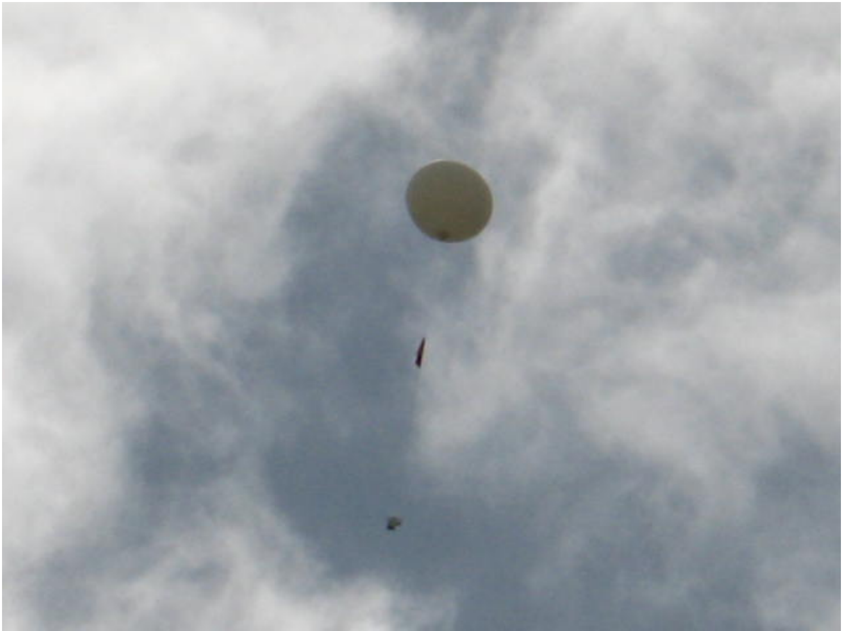
B5. Balloon with radiosone and GPS receivers
