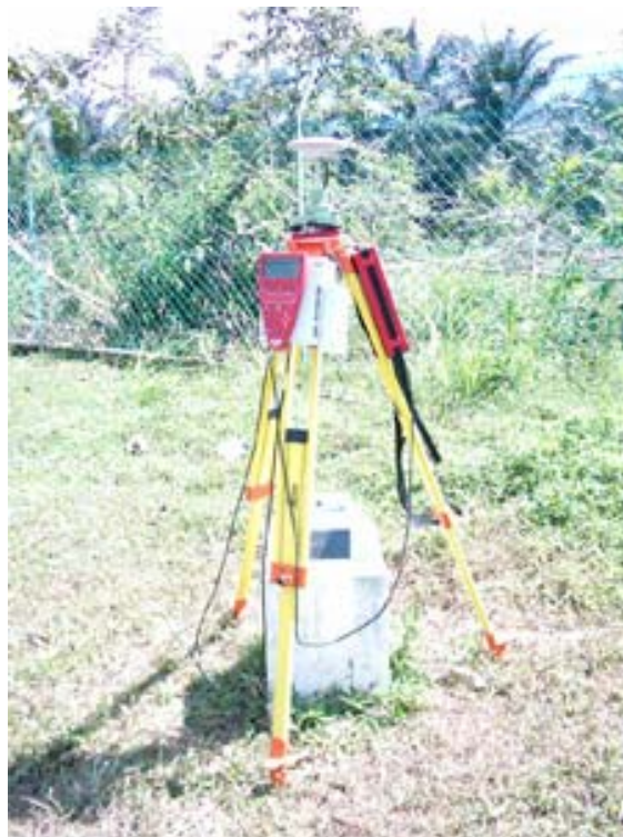
Figure 3.4c: GPS receiver over GPS control point
