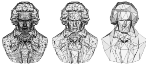
Figure 3.1 Three levels of detail of the Ludwig model. Left, 4998 faces; center, 1250; right 250 faces (Ribelles, et al. 2001)
