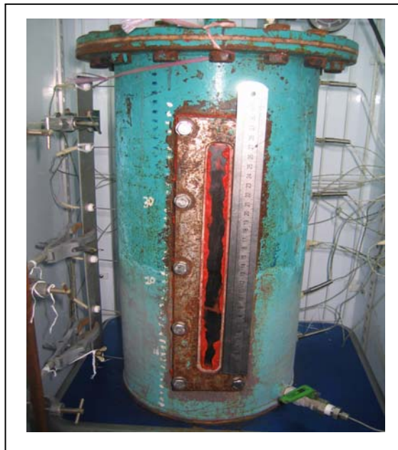
Figure 4.16: The Early Stage of Ice Layer Formation Due to Condensation of Water Vapor
