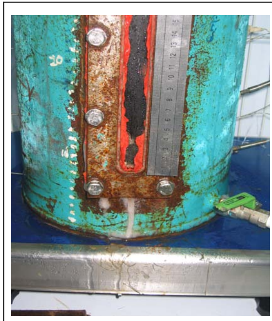
Figure 4.18: Liquefaction of Ice Formation Layer
