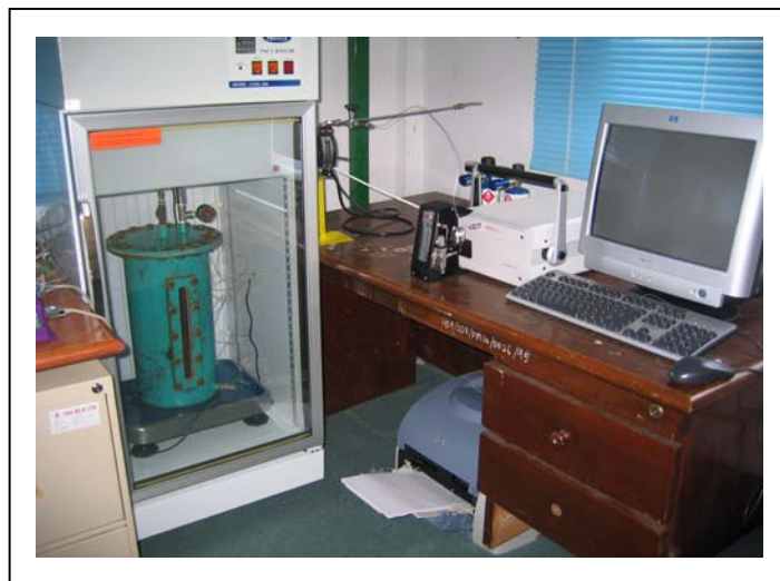
Figure 3.6. Arrangement of On-line Gas Chromatography
