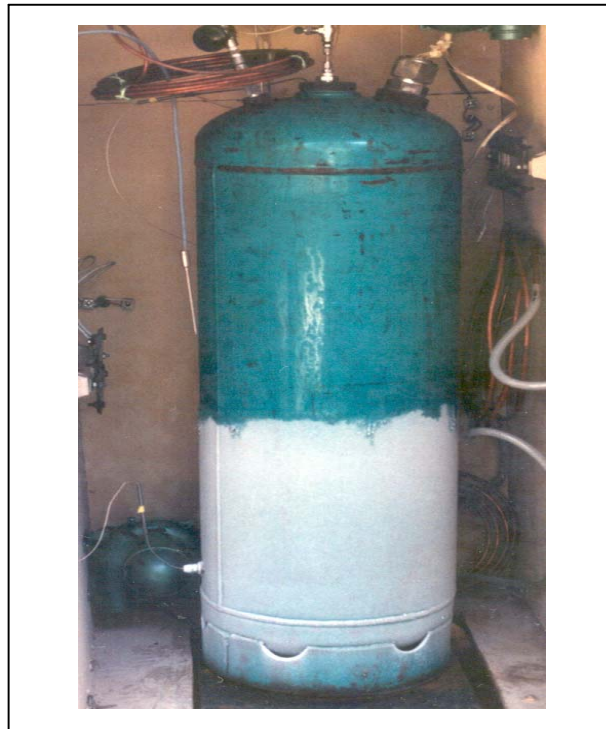
Figure 2.17: Ice Layer on the Outer Cylinder Wall
