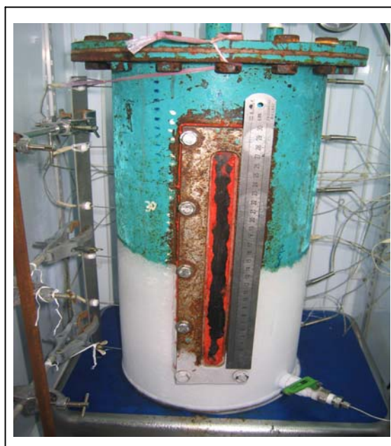
Figure 4.17: Final Stage of Ice Formation Layer
