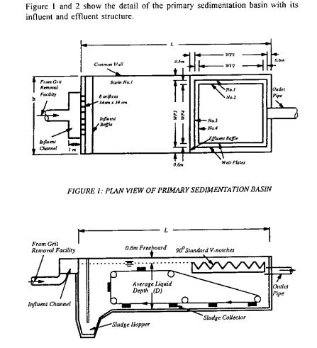
FIGURE 2: LONGITUDINAL SECTION OF PRIMARY SEDIMENTATION BASIN
