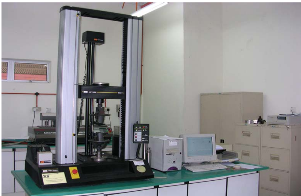
Figure 3.8: Instron universal tensile machine model 5567
