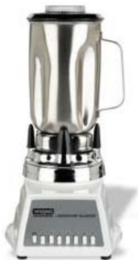
Figure 3.1: Laboratory scale Fielder mixer
