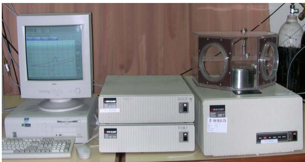
Figure 3.14: Perkin Elmer Differential Scanning Calorimeter Analyses
