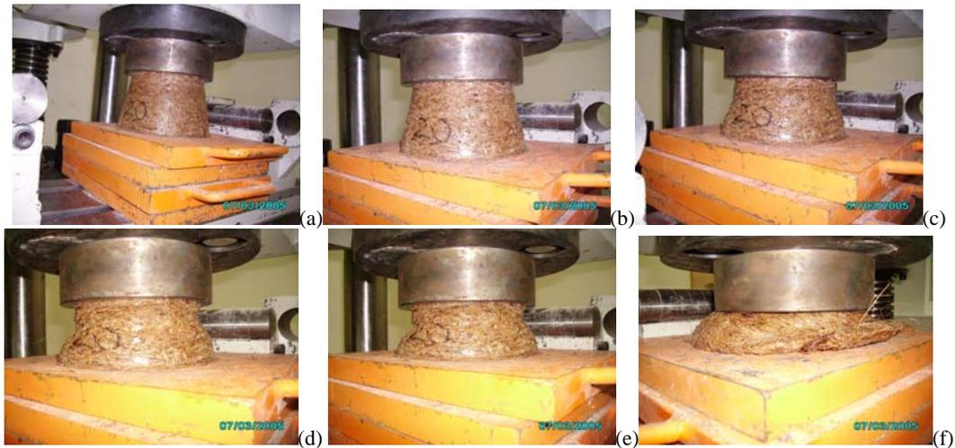
Figure 5 The sequence of cone deformations under axial compressive loading (vertex angle  $5^\circ$  and 20% fiber volume fraction).
