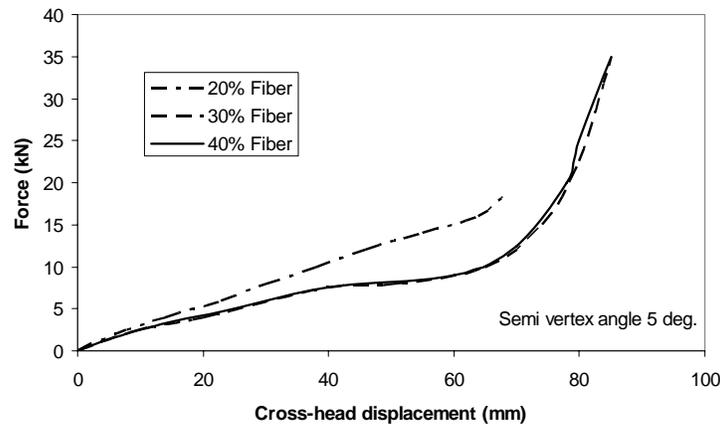
Figure 2 Force-displacement curves of conical composite with semi-vertex angle  $5^{\circ}$  with different fiber volume fractions.
