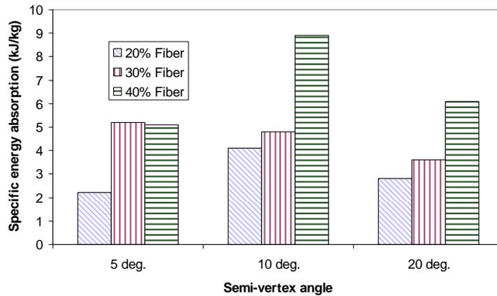
Figure 7 Specific energy absorption of conical composites.
