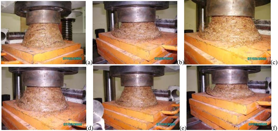
Figure 6 The sequence of cone deformations under axial compressive loading (vertex angle  $20^{\circ}$  and 40% fiber volume fraction).
