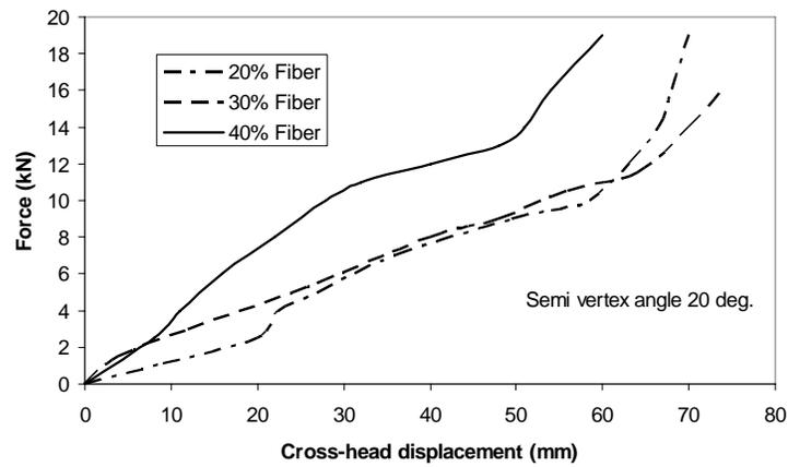
Figure 4 Force-displacement curves of conical composite with semi-vertex angle  $20^\circ$  with different fiber volume fractions.
