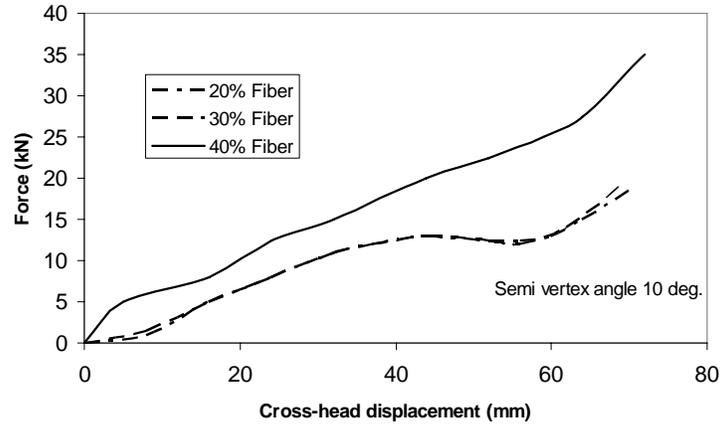
Figure 3 Force-displacement curves of conical composite with semi-vertex angle  $10^\circ$  with different fiber volume fractions.
