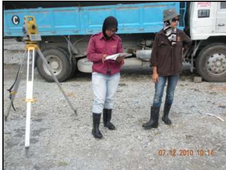
Figure 9: Topcon IS during scanning process
