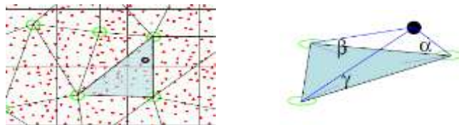
Figure 4: Point selection in ATIN filter is based on angle ( \alpha, \beta, \gamma ) and distance (Pfeifer, 2007)
