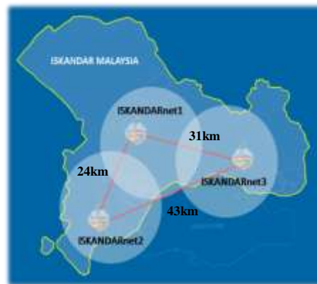
Figure 1: Network geometry of ISKANDARnet
