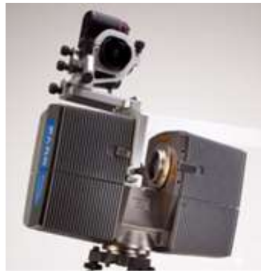
Figure 4: FARO Photon 120 integrated with Nikon DSLR 300s
