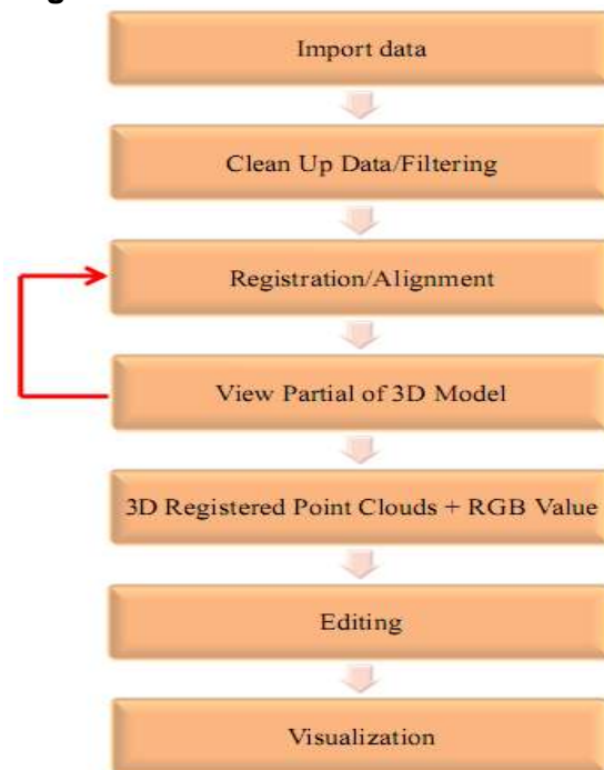
Figure 9: Point Cloud Processing Flowchart
