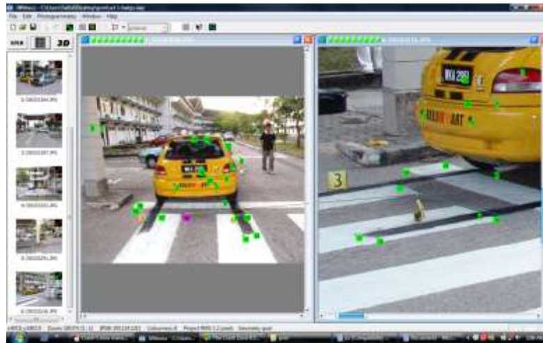
Figure 12: Image Referencing Using iWitness Software
