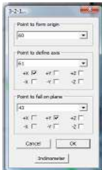
Figure 16: Process of Assigning Coordinate Axes
