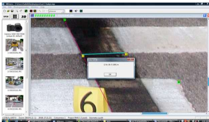
Figure 21: Example of a Non-Contact Measurement Using iWitness on Width of Tyre
