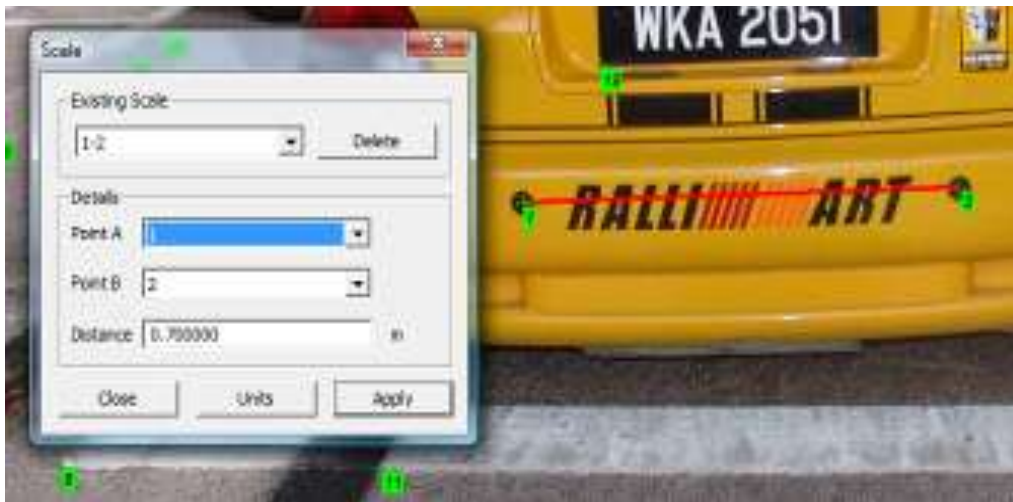
Figure 15: Process of Assigning Scale
