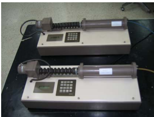
Figure C1: Two independently controlled water pressure systems, giving maximum pressure up to 1000 kPa used for hydraulic consolidation and permeability tests in laboratory
