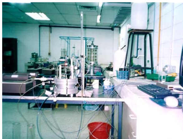
Figure C9: A burette connected to Rowe consolidometer for hydraulic permeability test
