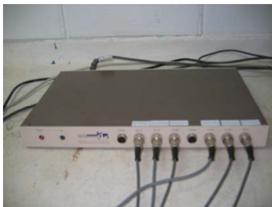
Figure C2: Power supply and readout unit for the electric pore pressure transducer
