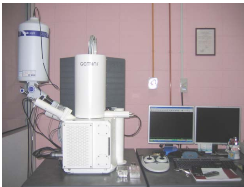
Figure B2: The equipment for SEM test.
