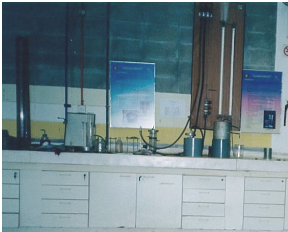
Figure F3: Constan Head Permeability Test
