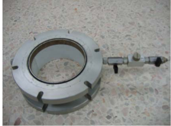
Figure C6: Rowe cell body of 151.4 mm internal diameter
