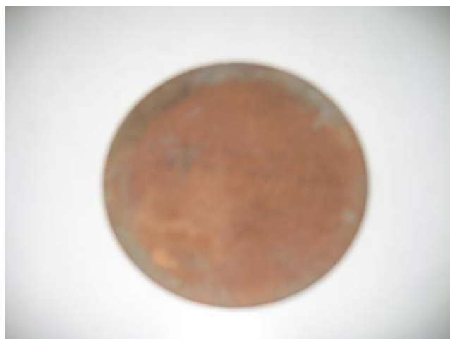
Figure C4: Sintered bronze disc of 4 mm thickness
