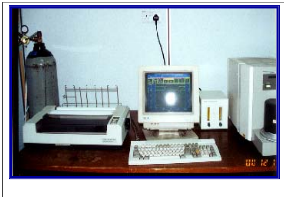
Figure 3.7 : Differential Scanning Calorimetry (DSC)
