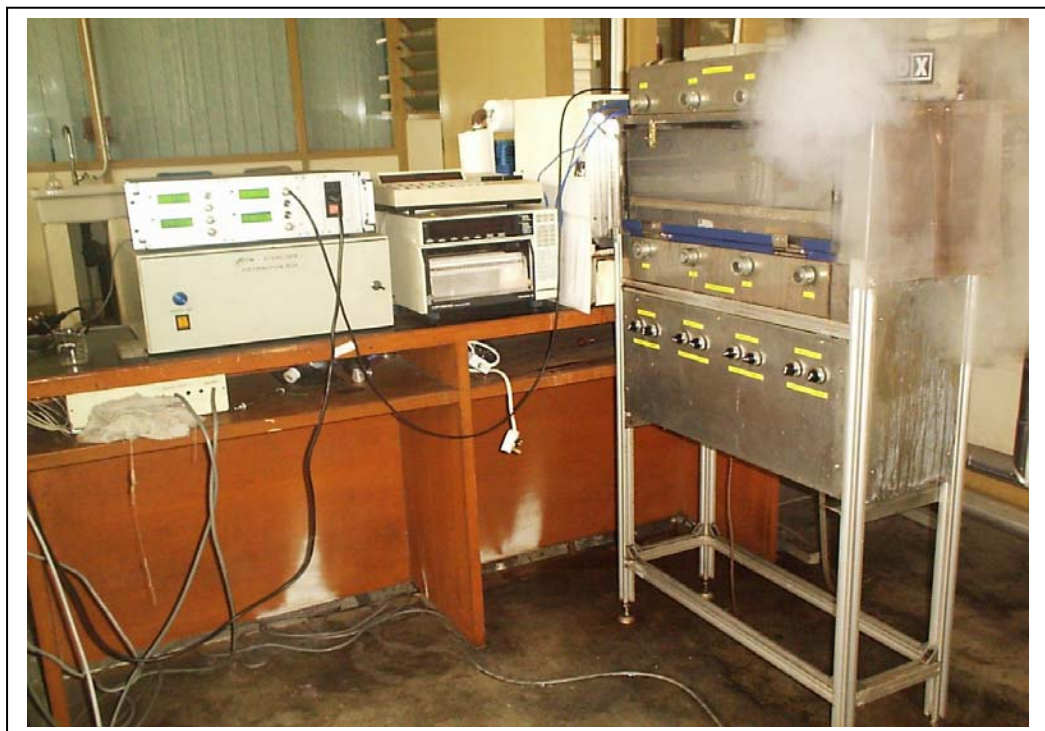
Figure 2.2: Profiler of the Sterilizer with an Air Curtain and Sensor Attachment Set-Up
