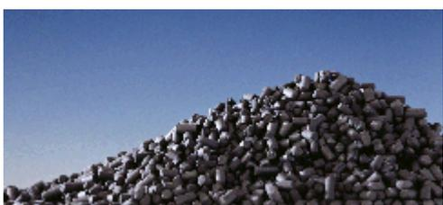
**Figure 2.5: Pelleted activated carbon (Chemiviron, 1998)**
