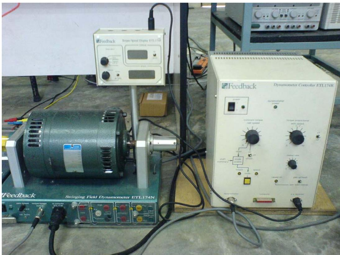
**Figure 4.9:** Dynamometer and the dynamometer controller
