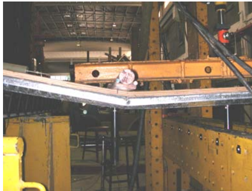
Fig. 9 Permanent bend of plywood and steel deck
