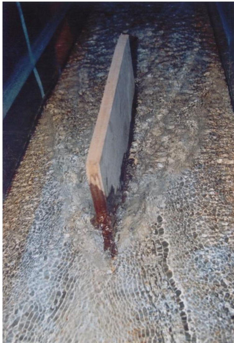
Figure 4.64 Run up at rectangular nose of wood pier
