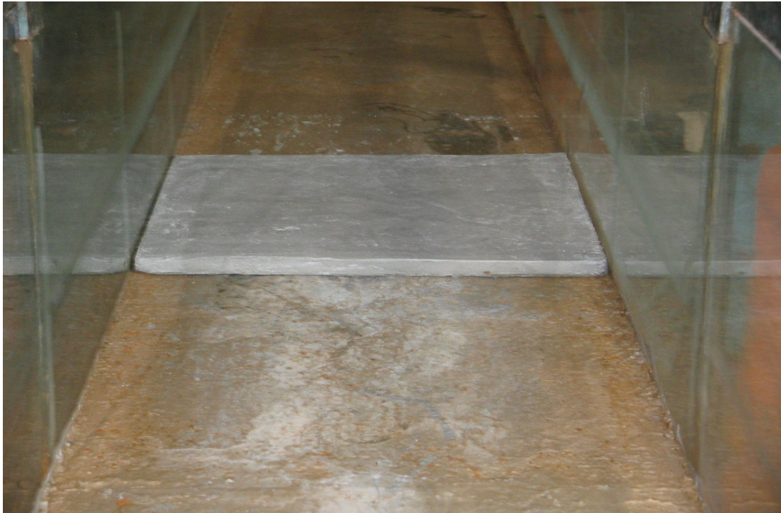
Figure 4.12 Front view of mortal weir
