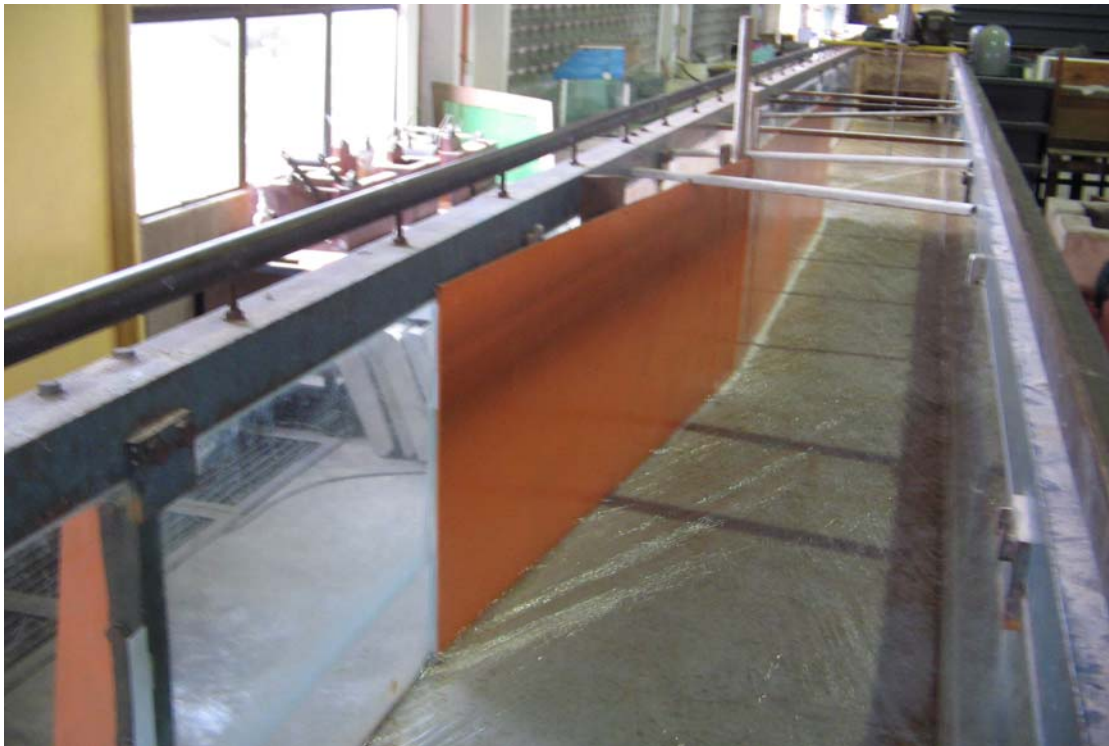
Figure 3.8 Contraction & 90 degree expansion test case
