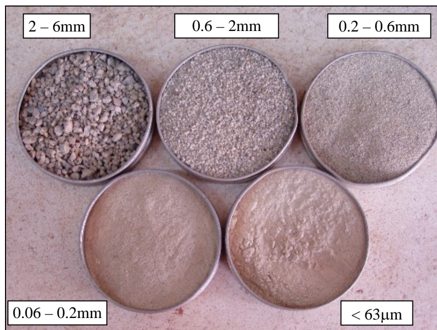
Figure 4.4: Infill sample divided according to the grain size
