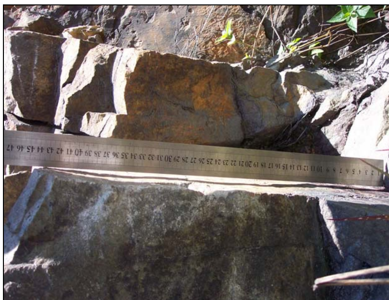
Figure 3.4: Measuring of JRC
