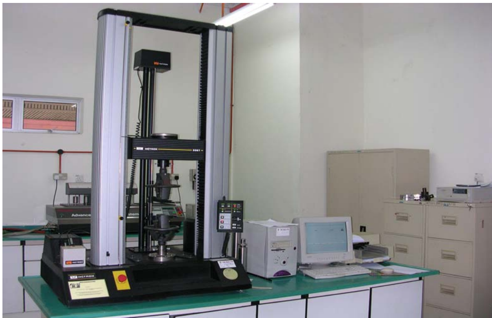
Figure 3.8: Instron universal tensile machine model 5567
