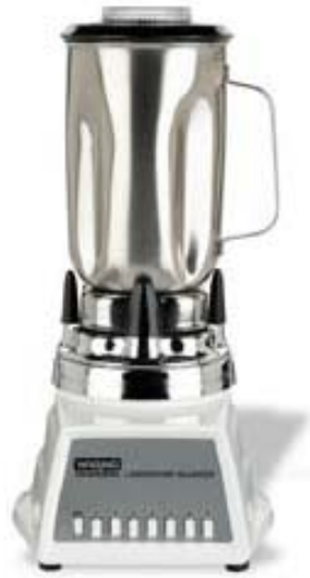
Figure 3.1: Laboratory scale Fielder mixer
