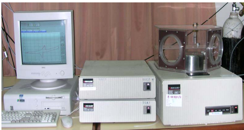
Figure 3.14: Perkin Elmer Differential Scanning Calorimeter Analyses
