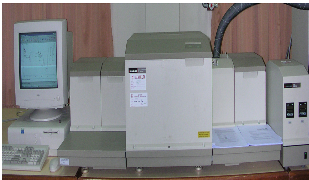
Figure 3.13: Perkin Elmer Spectrum 2000 Explorer FT-IR Spectrometer
