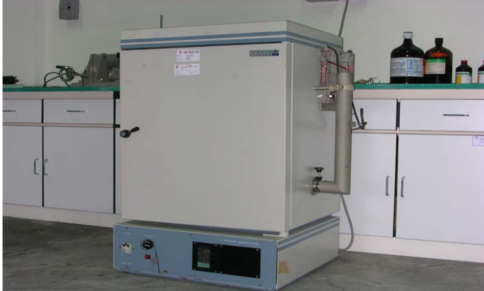
Figure 3.9: Ceast heat aging oven type 1175
