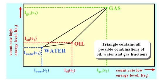
Figure 2: Graphical representation of measurement results of dual energy gamma ray on wet gas fluid [9]
