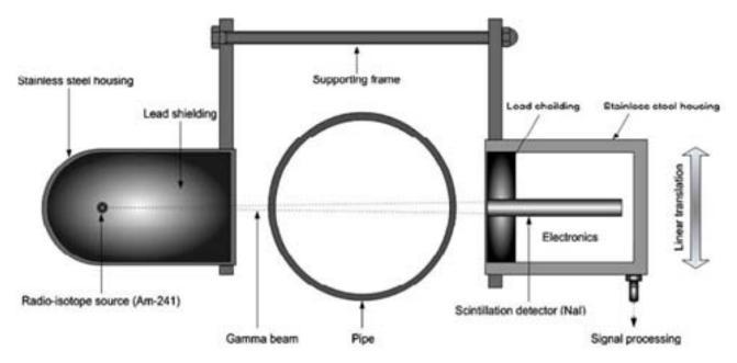
Figure 3: (a) Different elements of radio-active measuring method in wet gas flow meters [11]
