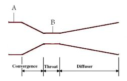
Figure 1: Cross Section of Venturi flow meter
