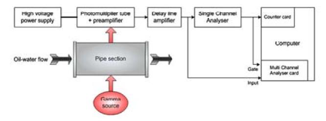
Figure 3(b): Block diagram of radio-active measuring method in wet gas flow meters [11].
