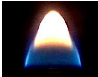
Figure 4.1: A low velocity stationary nonpremixed flame. V = 0.2 cm/s, \omega = 0
