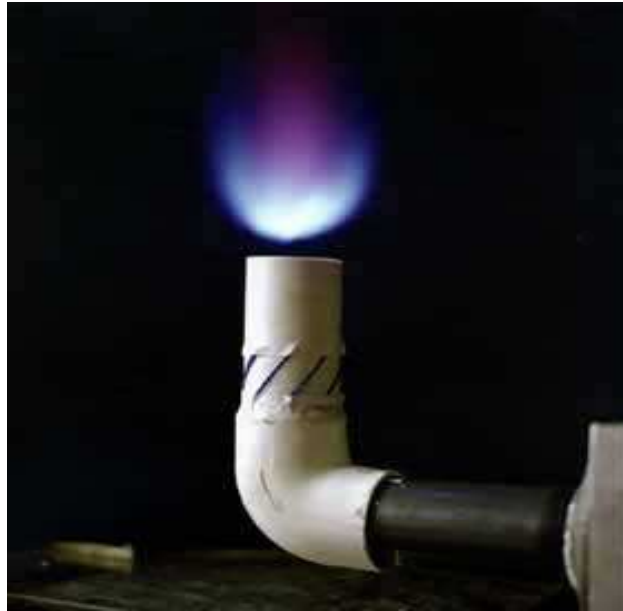
Figure 1.4: Sample of flame from tangential entry swirl burner [42].
