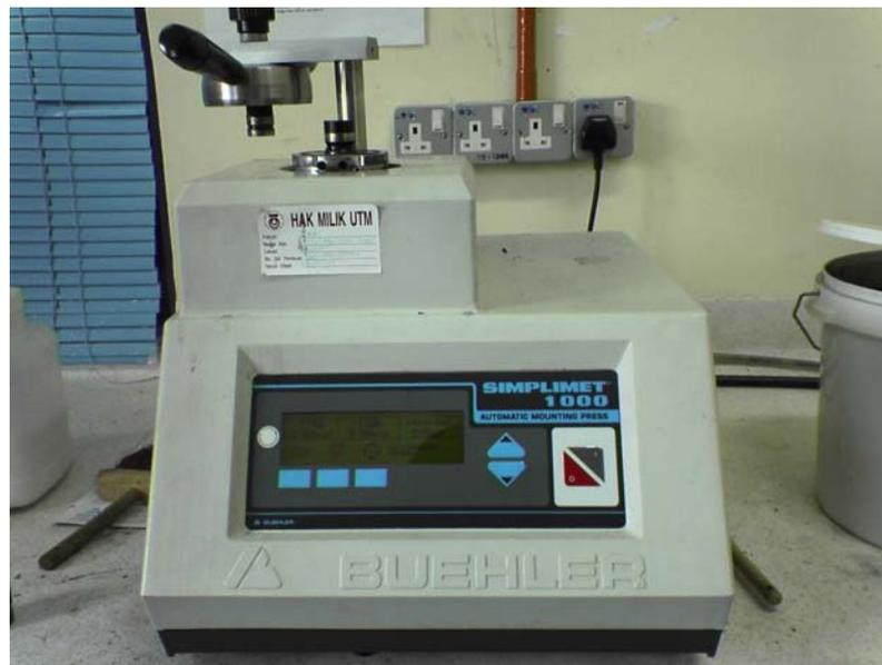
**Figure 3.12** The mounting equipment
