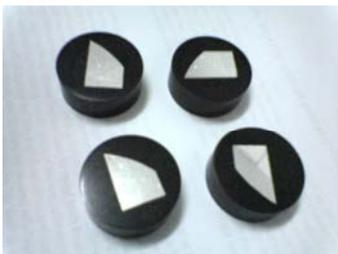
Specimens for the microstructure observation and Vickers Hardness Test
