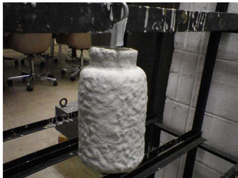
**Figure 3.5** Mould with 5 layers
