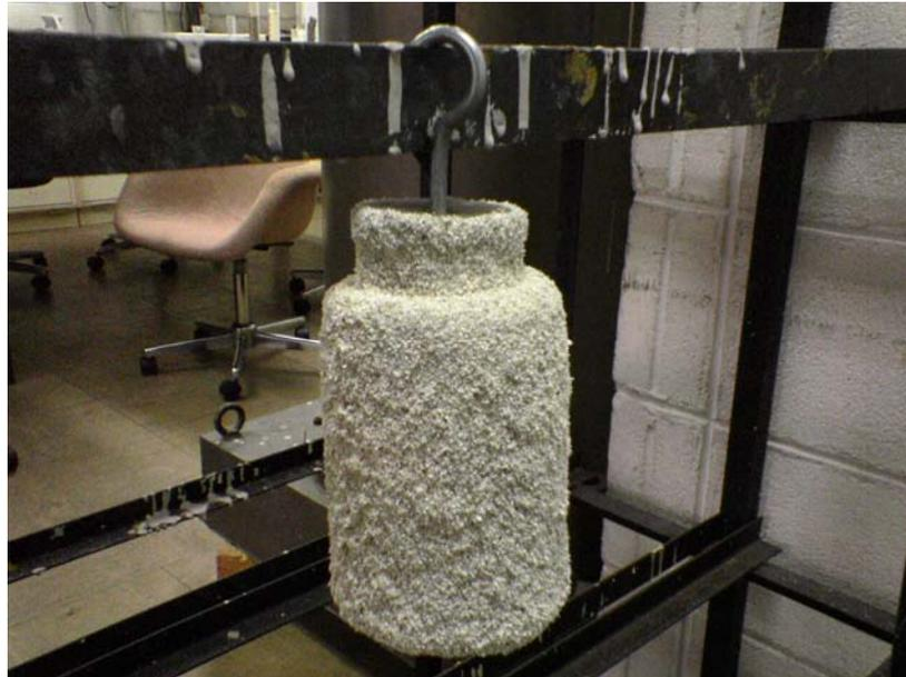
**Figure 3.4** Stucco systems for the mould with 5 layers
