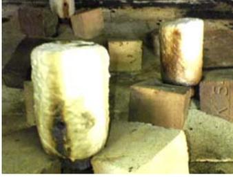
Wax melted out from the mold material in the dewaxing stage
