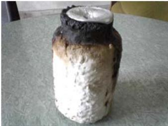
Mold material with solidified aluminium alloy
