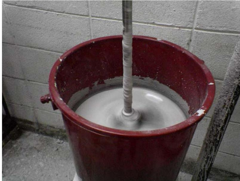
**Figure 3.3** The mixture of the slurry
