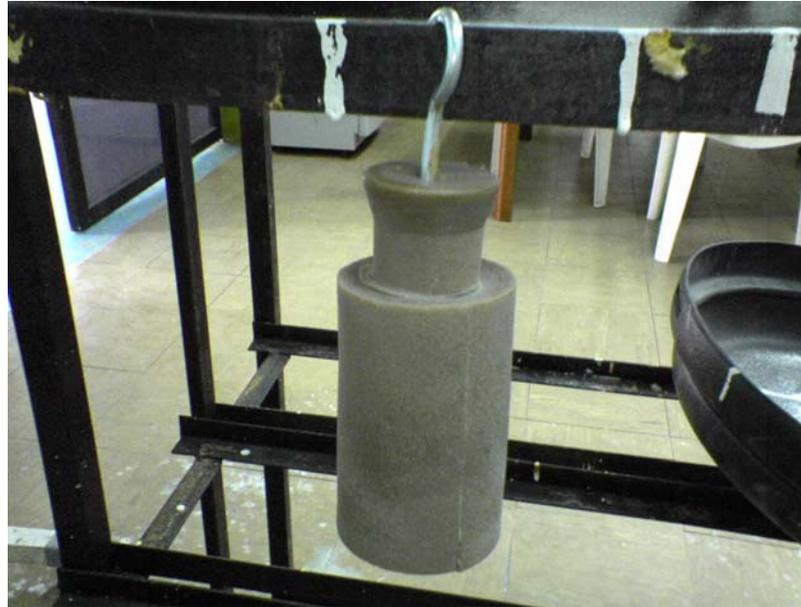
**Figure 3.2:** Pattern after sand blasted.
