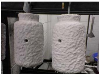
A hole is drilled to locate the thermocouple in order to measure the inner wall temperature
