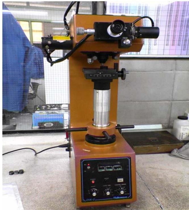
**Figure 3.14** Vickers Hardness Tester
