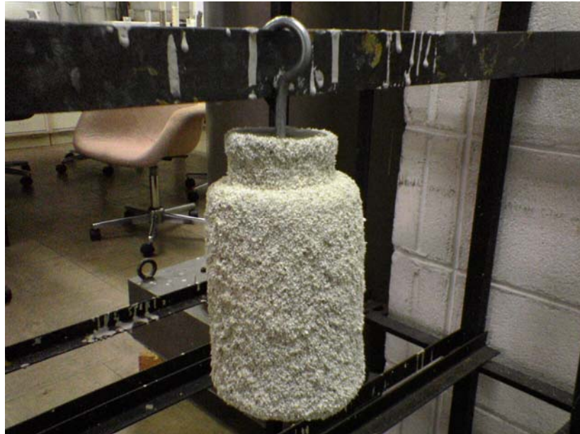
Figure 3.4 Stucco systems for the mould with 5 layers
