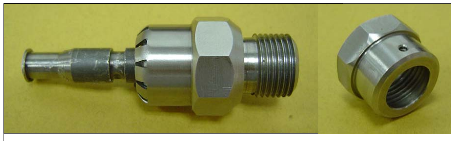
Figure 6.11: (Left) sub-assembly of injector Body (CBDY-0100) + Solenoid (CSNDA0100), and Lock (PLCK-0100)
