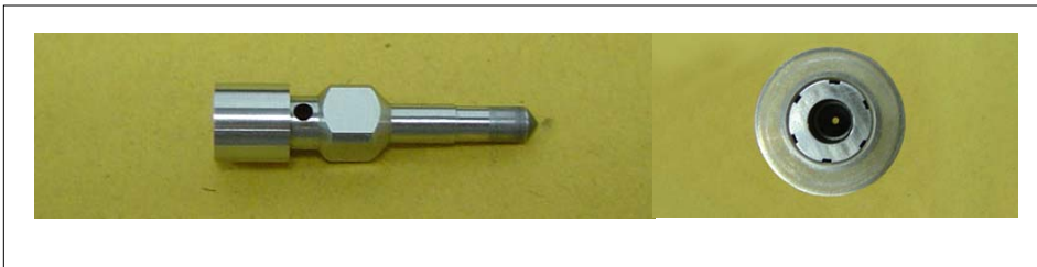
Figure 6.10: (Left) Needle (PNDL-0100), sub-assembly of Nozzle + Swirler
