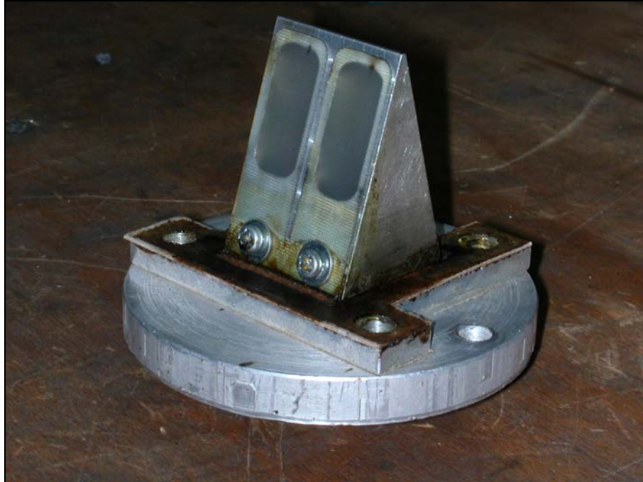
Figure 9.25: The reed valve of the main induced port
