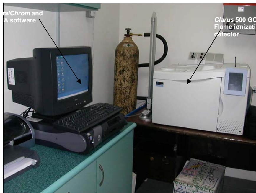
Figure 13.59: Hydrocarbon gas chromatography set-up
