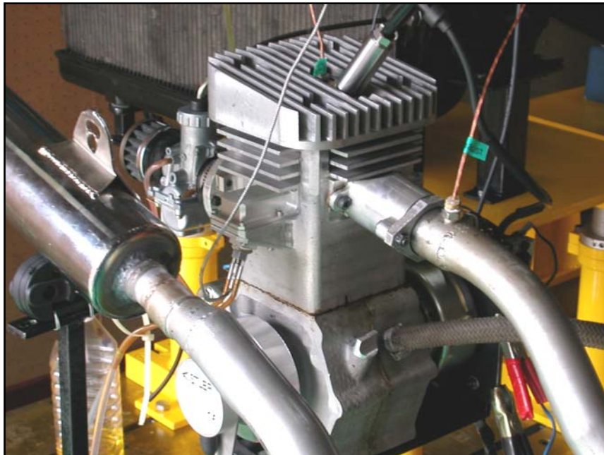
Figure 13.4: The engine on stand with thermocouple fitted onto the exhaust pipe
