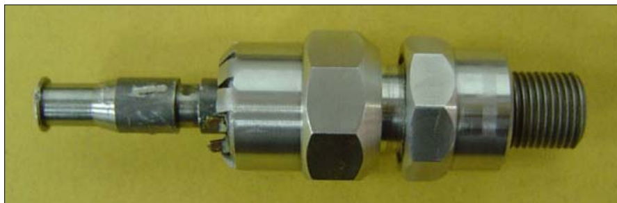
Figure 10.7: Injector assembly (CINJ-0100)
