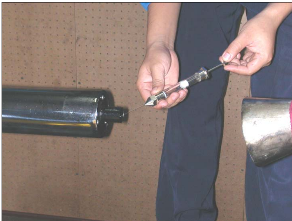
Figure 13.61: A syringe (of 20 ml) was used for collecting samples from the gas stream of the engine tail pipe
