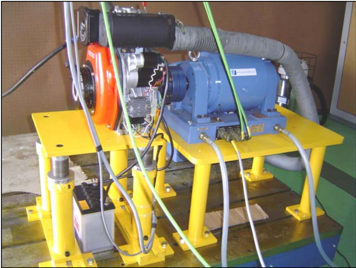
Figure 13.1: The Magtrol 30kW capacity engine testbed
