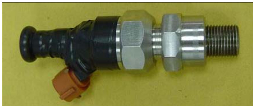
Figure 10.6: Injector assembly (CINJ-0100) + wire harness + o-ring
