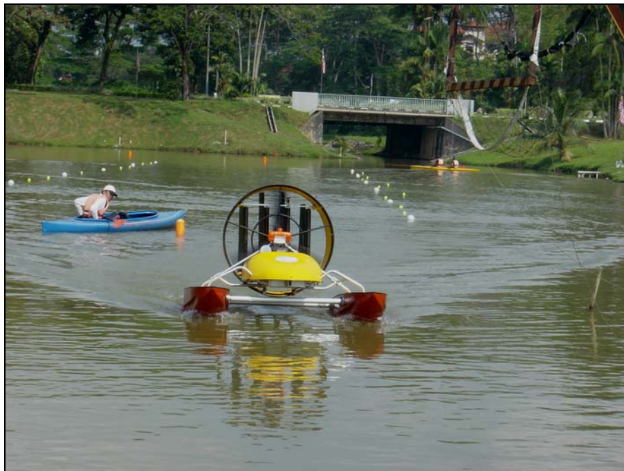
Figure 13.65: The engine and the unmanned surface craft on trial
