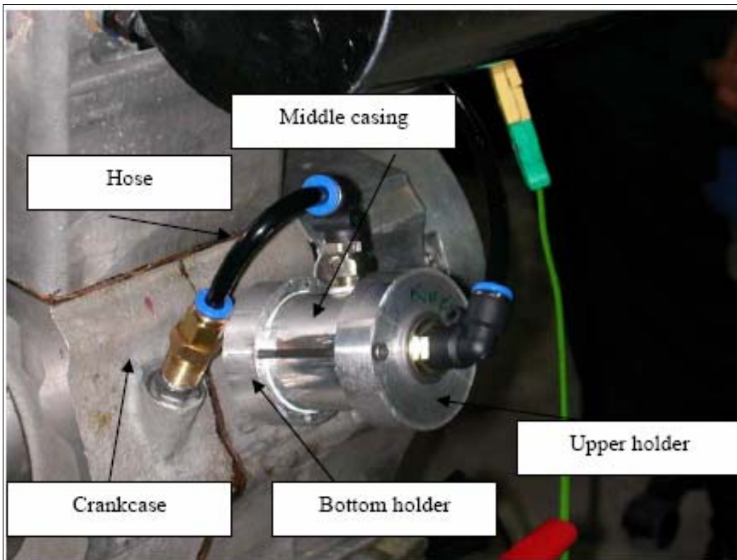
Figure 5.17: The engine breather system fitted onto the engine
