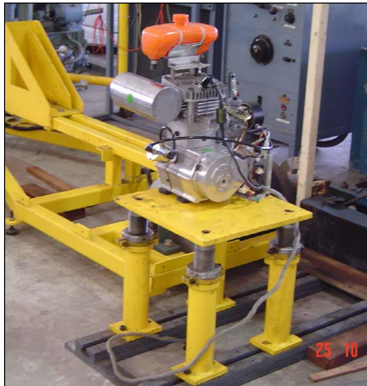
Figure 13.18: Two-Stroke Gasoline Engine undergoing noise and vibration evaluations.
