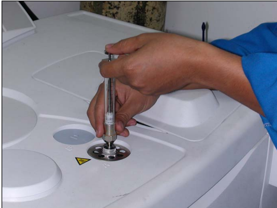
Figure 13.62: The injection of a sample into the column for detection.
