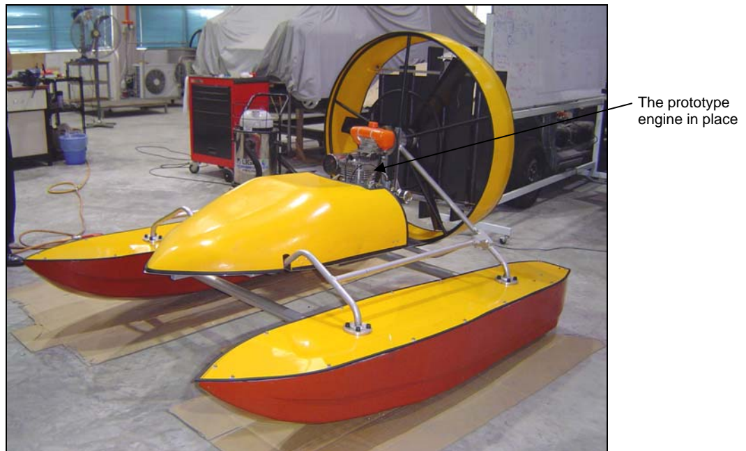
Figure 13.63: Mounting of the prototype engine onto a remotely piloted water surface craft
