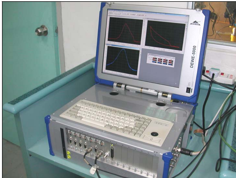
Figure 13.6: The Dewetron 2000 High-speed data acquisition system
