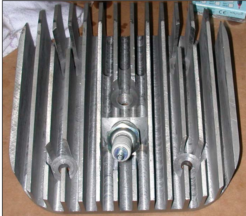
Figure 9.27: The area of the outer cooling surface
