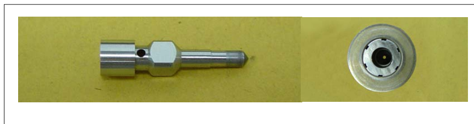
Figure 10.10: (Left) Needle (PNDL-0100), sub-assembly of Nozzle + Swirler
