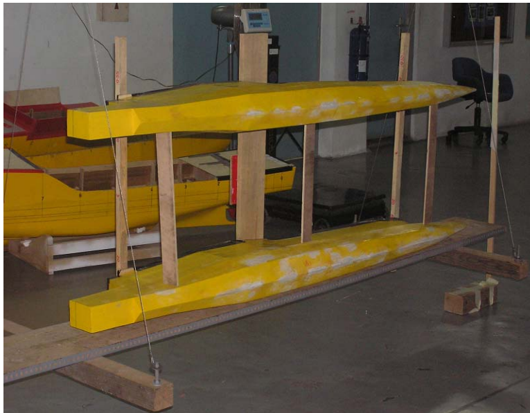
Photo 1: Side view of the model during the bifilar test
