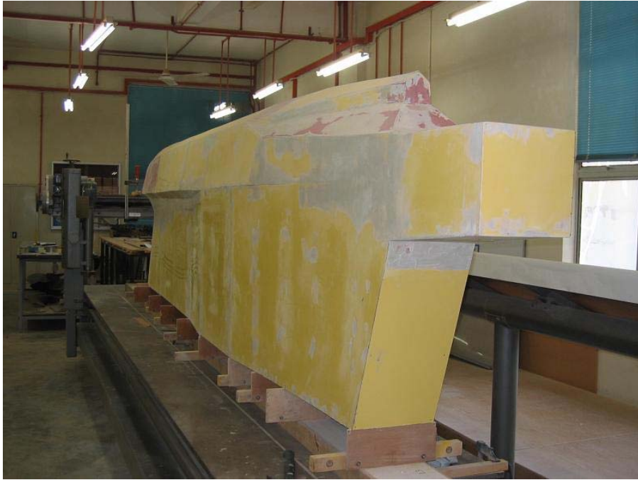
Figure 1: 6.0m length of Semi-SWATH prototype
