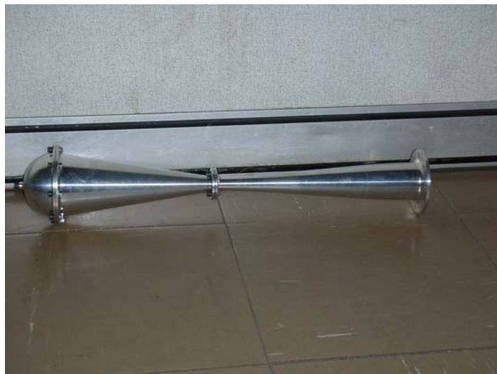
End Cap, Buffer and Small Diameter Resonator
