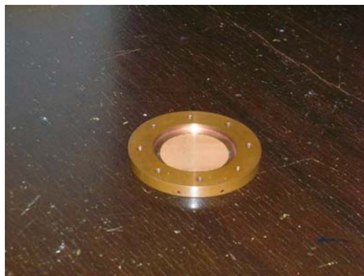
Cold Heat Exchanger
