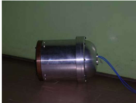
Driver Housing, Driver Cap, Large Diameter Resonator Hot Heat Exchanger
