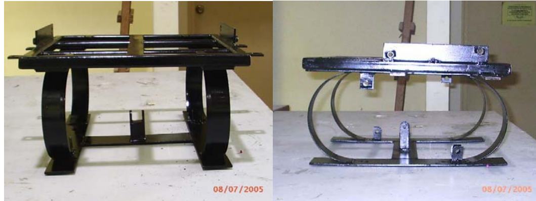
Figure B12: New seat structure (without absorbers)
