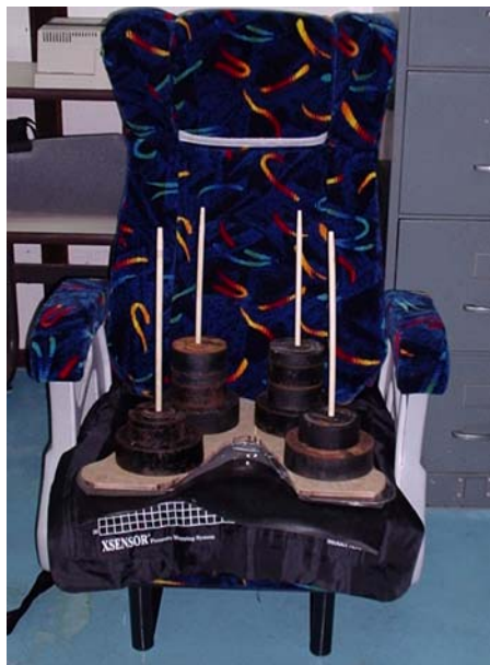
Figure 4.5: Rigid Load Dummy to determine the correct pressure distribution for vibration test
