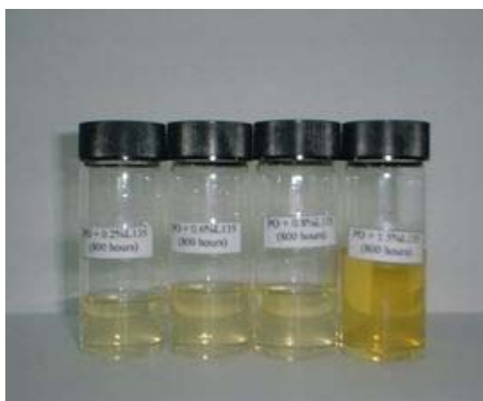
Figure 4.51b: Appearance of palm oil with additive L135; from left: 0.2%L135, 0.6%L135, 0.8%L135 and 1.5%L135 (800 hour).
