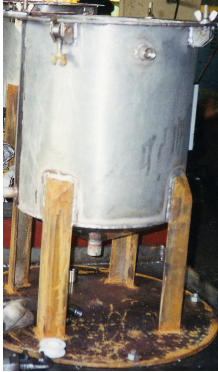
Figure B3: Fabrication of hydraulic reservoir.
