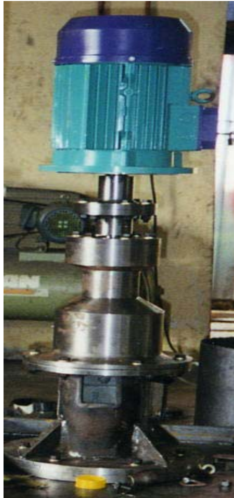
Figure 3.5: Photograph of pump-motor assembly.
