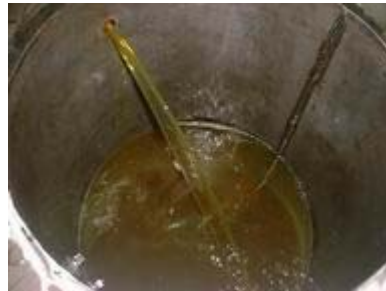
Figure 4.23: Bubbling and aeration in hydraulic system.
