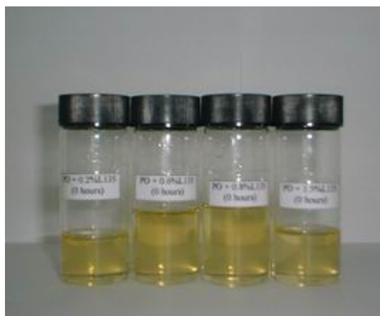
Figure 4.51a: Appearance of palm oil with additive L135; from left: 0.2%L135, 0.6%L135, 0.8%L135 and 1.5%L135 (0 hour).
