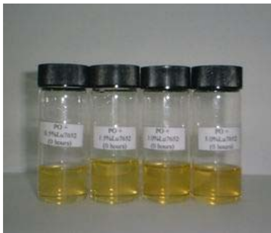
Figure 4.52a: Appearance of palm oil with additive Lubrizol 7652; from left: 0.5%Lubrizol 7562, 1.5 %Lubrizol 7652, 2.0%Lubrizol 7562 and 3.0%Lubrizol 7652 (0 hour).
