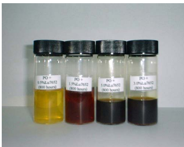
Figure 4.52b: Appearance of palm oil with additive Lubrizol 7652; from left: 0.5%Lubrizol 7562, 1.5 %Lubrizol 7652, 2.0%Lubrizol 7562 and 3.0%Lubrizol 7652 (800 hour).
