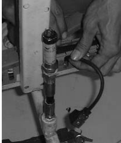
Figure 3.7b: Pressure transducer installation via flexible adapter.
