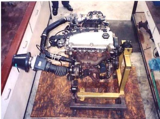
**Fig. 3.12:** 4G92 engine with complete turbo kit installed.
