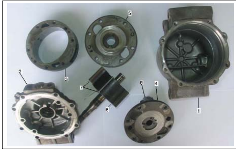
Appendix C1: Dismantled component of Patco compressor
