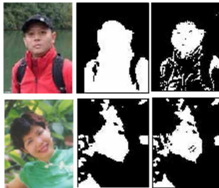
Figure 7 Skin Detection on Sample Images from the WWW Database using Threshold Technique (Center) and Neural Network (Right). (J. Dargham et al., 2004)
