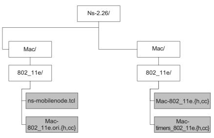
Figure 5 The files in ns-2 framework that are edited and added
