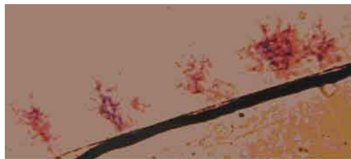
Figure 1.5.2 Water trees in extruded insulation
