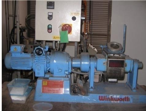
**Figure 5.1** Sigma type blade mixer
