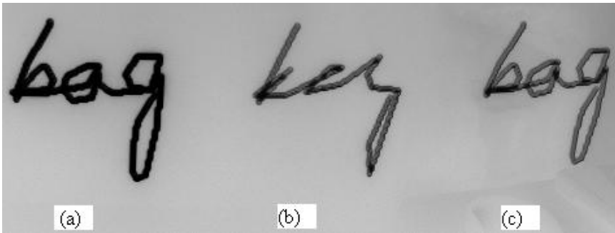
Figure 6 Filtering the data (a) original data (b) angular filtered data (c) cross-product filtered data
