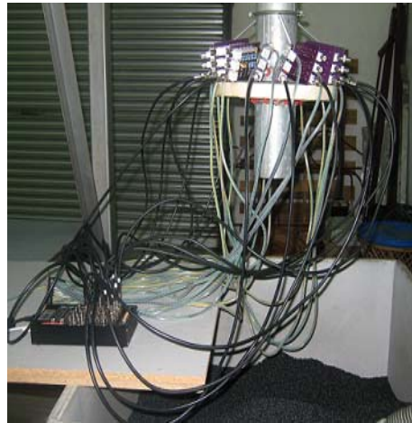
Figure 11.3 Measurement system of electric charge tomography
