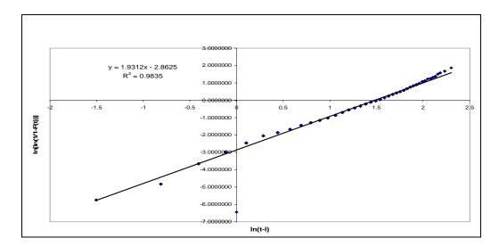
Figure 1: Weibull Probability plot of corrosion depth,  $T_6$
