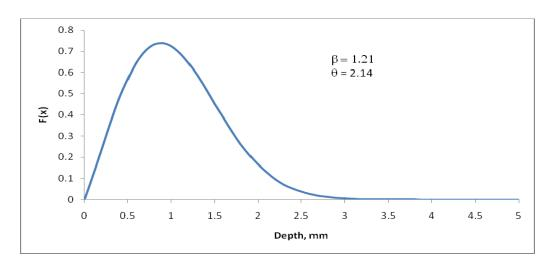
Figure 2: Weibull distribution of corrosion depth,  $T_6$
