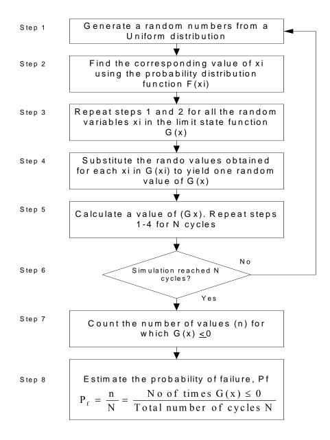
Figure 3: Procedure of failure probability estimation using Monte Carlo simulation method.
