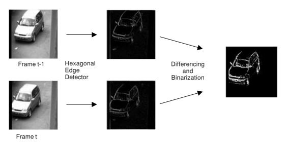
Figure 2 Moving edges extraction process
