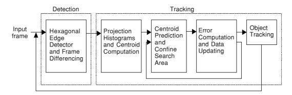
**Figure 1** The proposed detection and tracking algorithm
