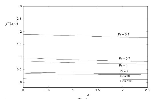
**Figure 7** Variation of the surface shear stress (f''(x,0)) with x for exponential variation in surface heat flux and various Prandtl number, Pr
