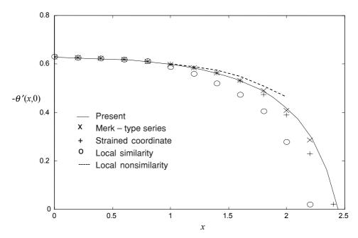
Figure 2 Comparison of dimensionless temperature gradient for sinusoidal variation in wall temperature (Pr = 0.7)
