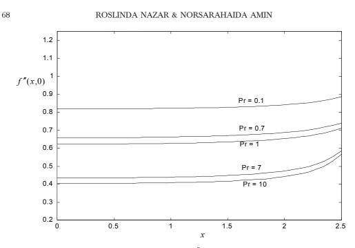
**Figure 3** Variation of the surface shear stress (f''(x,0)) with *x* for sinusoidal variation in wall temperature and various Prandtl number, Pr
