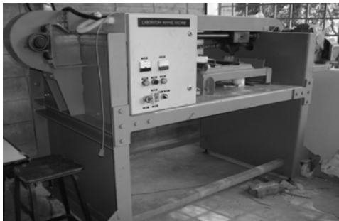
Figure 5 : Laboratory ripping machine rock sample
