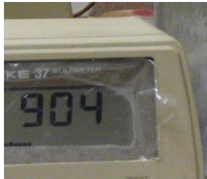
Figure 5: Example of the output voltage of boost converter at 904 V.
